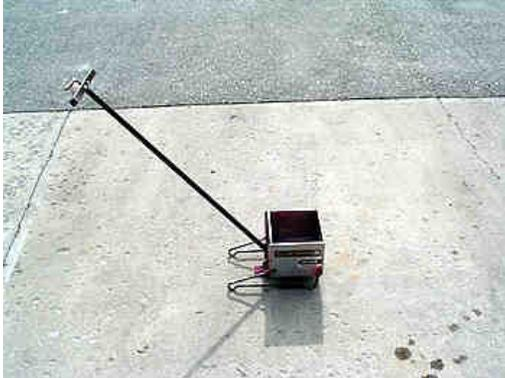
Tru Line Marker Tool is a commercial method of quickly and accurately putting down the circles for curling and hockey - although this takes practice to do “neatly”.
