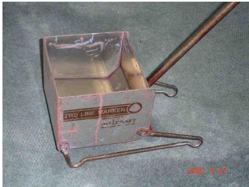
Tool is a metal box with thin slot inside where a brush assembly is attached allowing paint to seep down brush bristles and make a 2” wide line. Box sits on wire runners.
