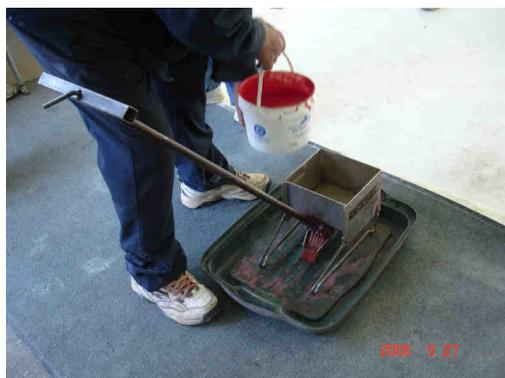
Fill reservoir with ice paint. Plunger system in handle allows control of paint flow. A plastic lid or basin is handy to control spills or for moving Tru Line Marker into start position for each new circle.
