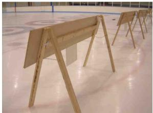
Cut two 2 x 4s in half, and put a hinge on the joint. The cross-mounted 2 x 4 provides added stability and stiffness.
